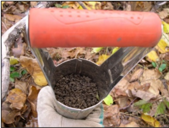
Figure 4. Soil corer (i.e. bulb planter) used to sample top 10cm of soil in treatment quadrats. (KRISTEN A. ROSS).
